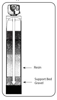
Fill tank one quarter full of water to protect distribution during gravel installation. Place the media into the tank in the order indicated above. Slowly and carefully add the gravel support bed and the filtration media leveling each layer as it is placed into the tank.
