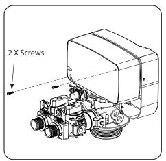
2. Remove two screws from the back of the valve cover
