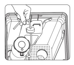
**6.** Take off the cover of the Res care bottle . Insert the wick, making sure it touches the bottom of the bottle. Insert the other end of the tube completely into the hole in the brine well cap. Automatic feeding will start in a few hours.
