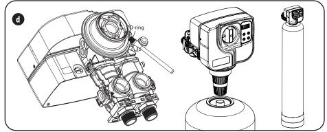
**d)** Unplug the riser tube, carefully position the valve over it and turn the valve into the threads in the fiberglass tank, tightening securely into tank. Note: Ensure that the internal O-ring in the valve fits securely over the riser tube. Silicone grease (part # 92360) or other food grade lubricant may be applied to the O-ring to ease installation of the riser tube.
