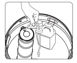
6. Take off the cover of the Res care bottle. Insert the wick, making sure it touches the bottom of the bottle. Insert the other end of the tube completely into the hole in the brine well cap. Automatic feeding will start in a few hours.
