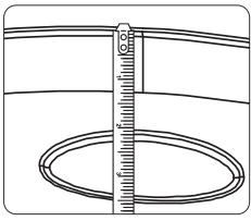
1. Install the grid and brine well inside the round tank. 2. Measure 2 inches from the top of the tank beside the oblong molding.
