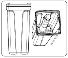
1. Install the grid and brine well inside the square tank. 2. Measure 2 inches from the top of the tank beside
