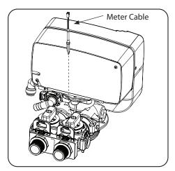
**1.** Disconnect the meter cable from the meter. (If flow meter is attached)
