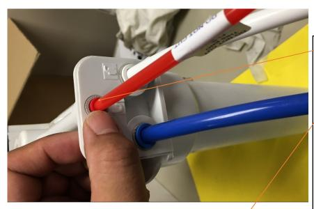
Remove the RED tubing from the RO Manifold and replace it with the New Flow Restrictor tubing supplied.
