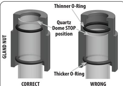
Quartz dome is past gland nut O-ring and is touching the inside top end of the gland nut. Caution: Do not push hard as it can break the quartz dome. Quartz dome is NOT past gland nut O-ring and is NOT TOUCHING the inside top end of the gland nut.
